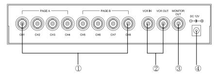
Fig. 2 (CONNECTION LOCATIONS - Rear View)
